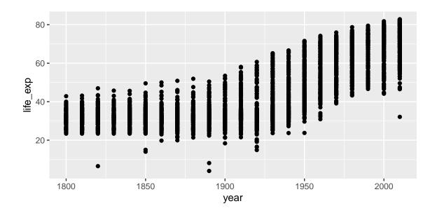
The call to ggplot and aes sets up the basics of how we are going to represent the various columns of the data frame. aes defines the "aesthetics", which is how columns of the data frame map to graphical attributes such as x and y position, color, size, etc. aes is another example of magic "non-standard evaluation", arguments to aes may refer to columns of the data frame directly. We then literally add layers of graphics ("geoms") to this.
