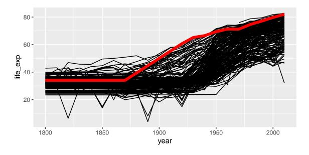
Notice also that the second <code>geom\_line</code> has some further arguments controlling its appearance. These are **not** aesthetics, they are not a mapping of data to appearance, but rather a direct specification of the appearance. There isn't an associated scale as when color was an aesthetic.
