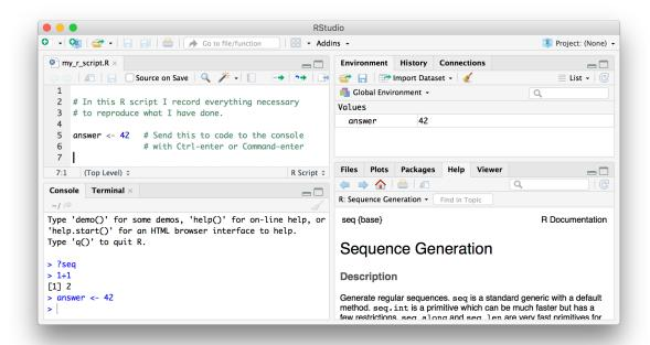
Open RStudio, click on the "Console" pane, type 1+1 and press enter. R displays the result of the calculation. In this document, we will show such an interaction with R as below.
